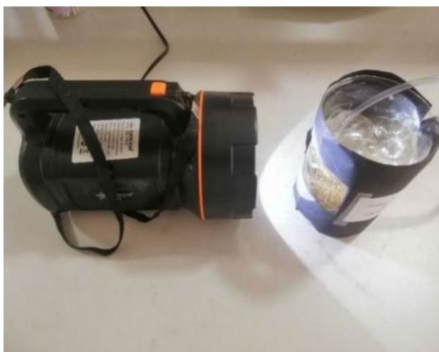
Fig. 3 Setup used for BSLA. After turn on the light source and, oxygen supply A. salina organisms were hatched after 24–48 h
