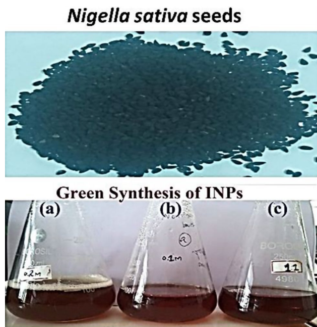
Fig. 1 Visual observation of black cumin extract mediated iron nanoparticles (a) 001:01 (b) 01:04 (c) 02:04
