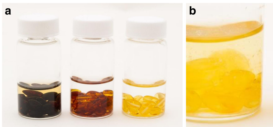
Fig. 3 Incubation of amber beads under various biologically relevant conditions. a Beads were removed from necklaces and sorted into colour variants, then stored at 37 °C in either pH 5.5 PBS or octanol for 6 months. Bead supernatants were periodically collected and succinic acid content was analysed by HPLC. b Succinic acid was only detected in the supernatant of light-coloured beads stored in octanol, in which one of three replicates had significantly fragmented and degraded
